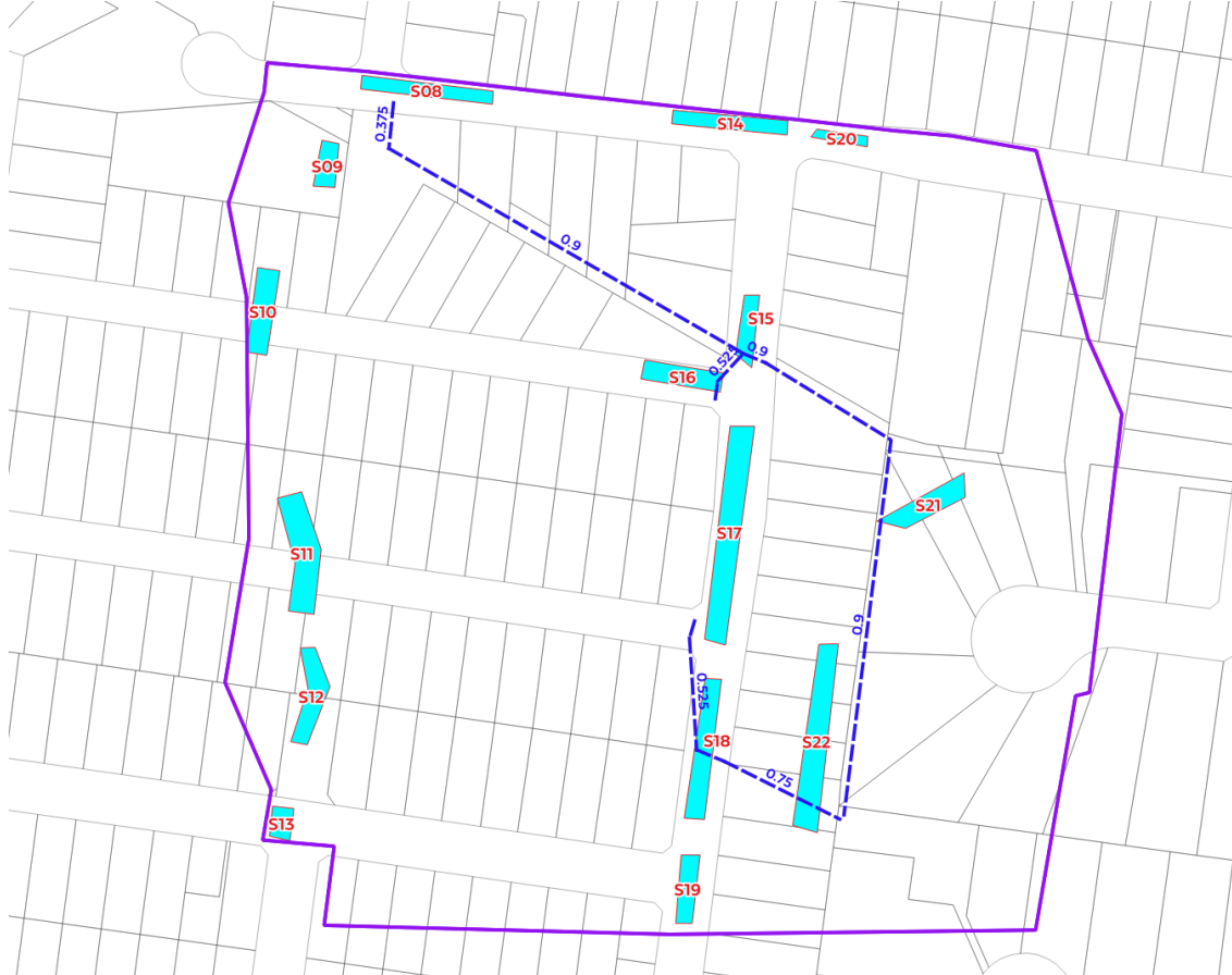
Figure 4.2: TUFLOW Extents & SA polygons & 1D network
